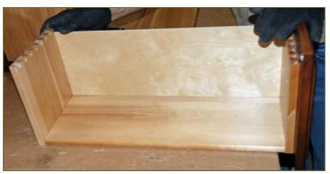
The front of the drawer box also has the Drawer Header attached. Apply glue lightly to the dovetail indentations of the drawer box front and lightly tap into place the side panel. Note: make sure the dado for the drawer box floor is aligned properly.
