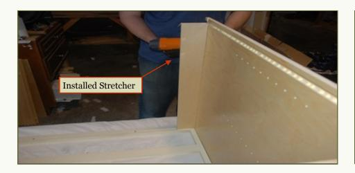
On Base cabinets install stretchers from front to back. These fit into the dadoes of the L & R side panels stiffening the cabinet and squaring the cabinet top,
