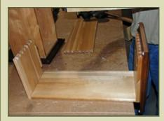
Then attach the dovetailed back panel in the same manner. Tack the dovetail with a pin nail to hold it together while glue sets.
