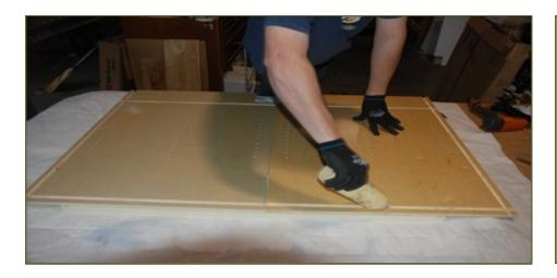
Lay Side panels (Left and Right Panels) on top of the face frame and apply glue to all dadoes.
