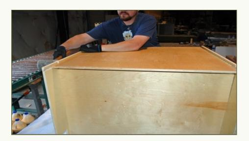
Prior to installing the back panel apply glue to all dadoes. Insert the back panel and lightly tap side panels to assure proper seating of panel into all dadoes, Pin nail the panel into place.
