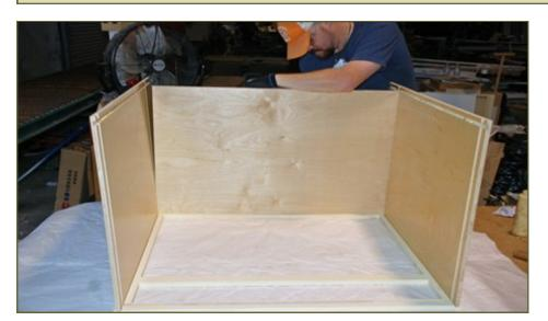
Inserting the Bottom Floor Panel.
